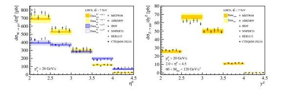
Figure 4.5: LHCb W/Z boson (pseudo)rapidity data. The left panel shows the  $W^{\pm}$  distributions in the pseudorapidity of the detected lepton compared to leading PDF sets. The right panel shows the Z in the rapidity of the resulting lepton pair. Figures from [239].
